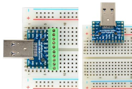
Figure 2: Examples of various methods for connecting the USB3-AM-BO-V1A to a breadboard
